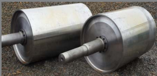
Turned drum with replaceable locking shaft
