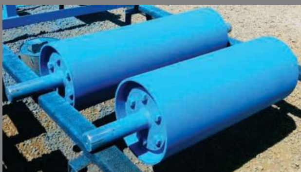
Turned drum with replaceable flanged shaft
