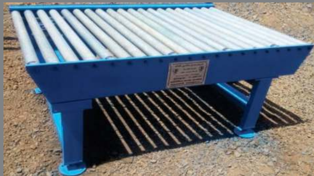
Electric roller table with bending sheet frame, galvanized roller and spiral gearbox
