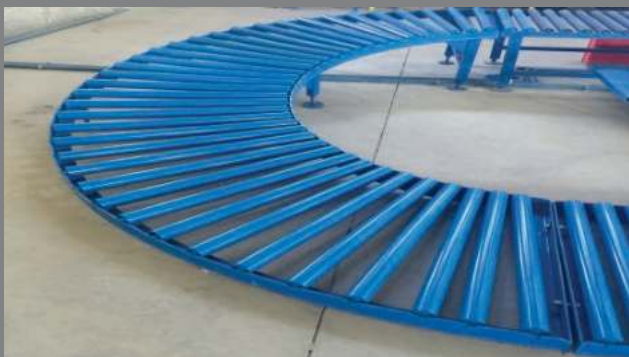
Manual roller table with 180 degree corner and corner frame
