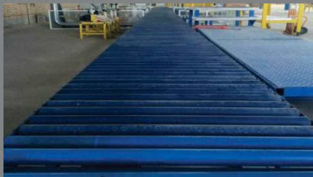
Manual roller table for home appliances assembly line
